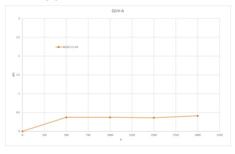
QUV using UVA 340 bulb, 8 hours 70°C, 4 hours 50°C condensation
