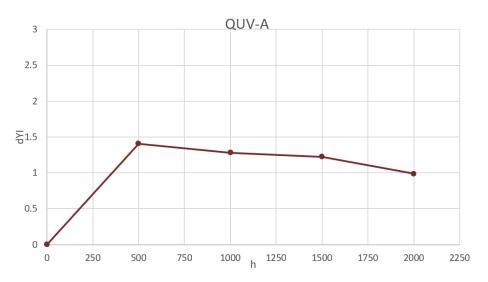
QUV using UVA 340 bulb, 8 hours 70°C, 4 hours 50°C condensation
