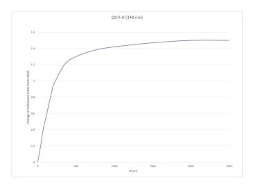
QUV using 340 bulb, 8 hours 70°C, 4 hours 50°C condensation
