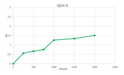
QUV using UVA 340 bulb, 8 hours 70°C, 4 hours 50°C condensation
