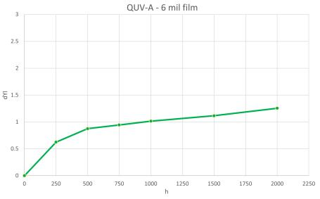
QUV using UVA 340 bulb, 8 hours 70°C, 4 hours 50°C condensation
