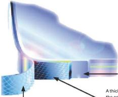
A thin layer of clear polyurethane film bonds Argotec Edge Seal to the glass laminate
